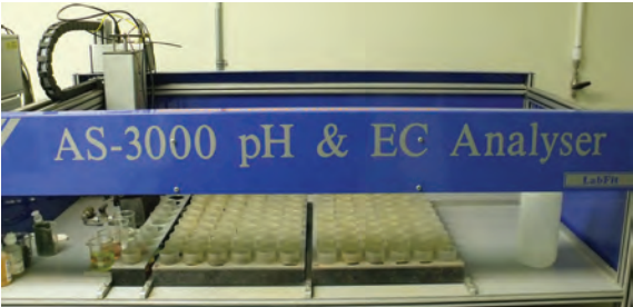
Soil testing labs like Western Soil Testing Labs in Parma, Idaho, have specialized equipment to measure salinity and other soil components.
